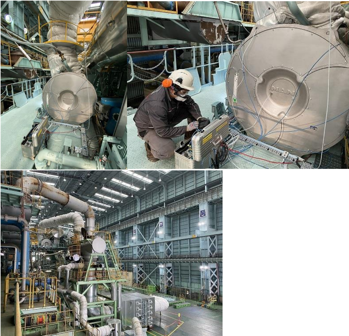
The PBST TCT60 type turbocharger pictured during the shop test at HSD Engine
