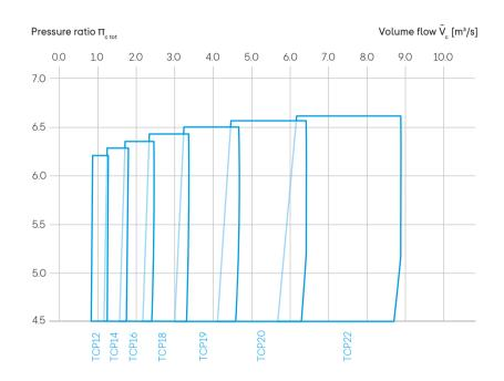
The TCP series of radial turbochargers can achieve maximum pressure ratios of up to 7, a benchmark figure that sets new industry standards. While existing 1-stage turbocharger systems typically deliver pressure ratios of well above 5, the TCP range achieves stable operating points of well above 6. These remarkable figures are thanks to a complete redesign of the aerodynamic stages on both the compressor and turbine side.
